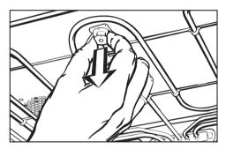
■ Pull down on the fixing knob for the element to release it.
